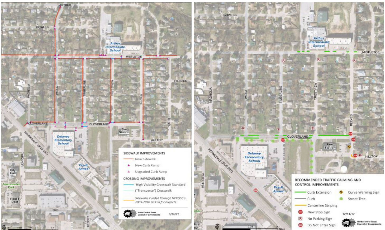
Figure 25: Pedestrian Improvements from 2017-2018 SRTS Project
