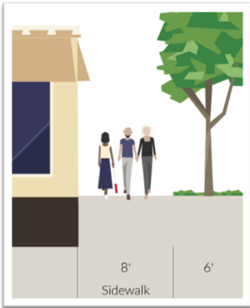
Figure 12. Example of acceptable sidewalk width & location along Link St
